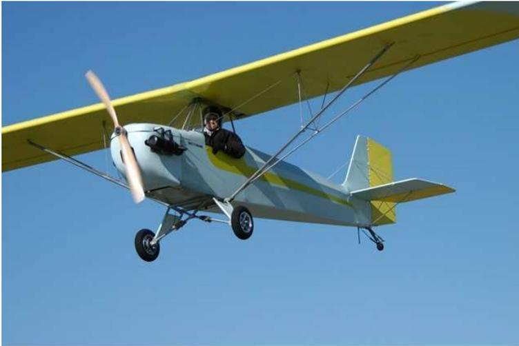
Unfortunately, no one identified this aircraft submitted by James Slade. It is the Fisher FP-505 Skeeter. The pylon-mounted high wing leaves the cockpit essentially unenclosed, offering the pilot spectacular visibility and the freedom of an open cockpit design. Fueled by a 40 horsepower Rotax, the compact FP-505 delivers plenty of go once you get up. Shock-absorbing gear and geodetic construction contribute to a sturdy aircraft in an exceedingly affordable price range.
