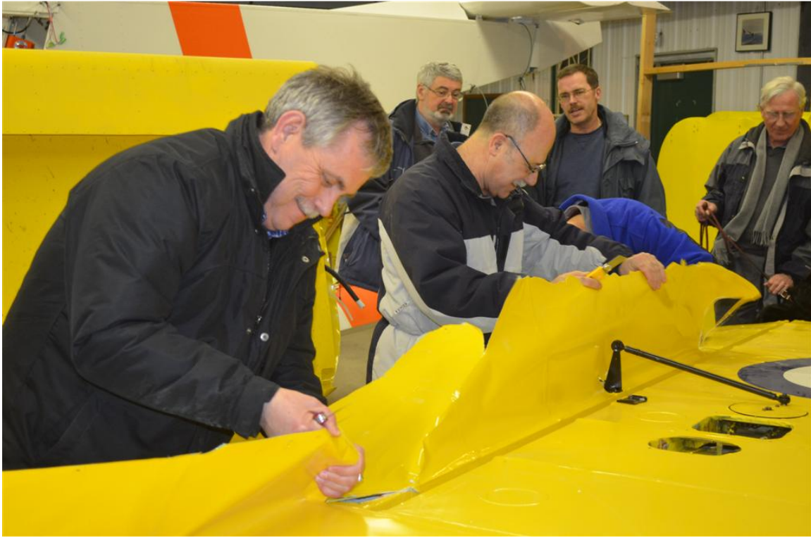
Volunteers work to remove the old fabric from the Tiger Moth wing
